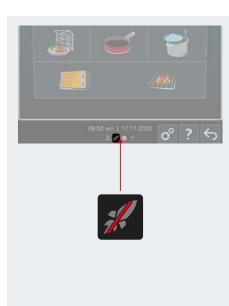
The iHexagon indicates whether microwave function is active or inactive using a rocket pictogram in the status bar. The function status display complies with safety-relevant specifications and authorization requirements.
