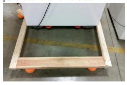
6. Slide unit off of the pallet jack into position on a sturdy level surface. Use stackers included if needed.
