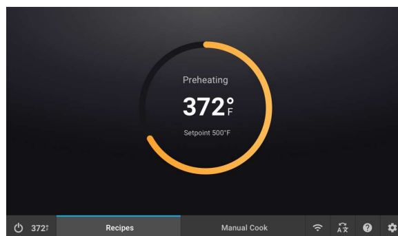
Figure 10: Oven Controls: OneTouch Preheat
