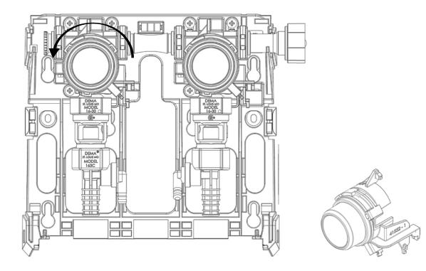
Step 3: In the interior of the button, you locate the locking tab. Break off the tab with pliers.
