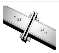
Then attach center support to the side supports. The bolts are packed in a red bag located in the center support carton.
