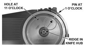
The Pin on the Knife Removal Tool fits the hole in the Knife at the 11 o'clock position.
