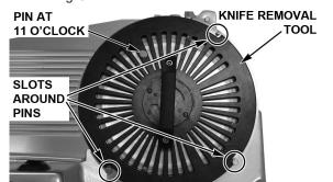
**NOTE:** If the Tool does not push the pins on the back of the Knife into the Hub, slightly nudge the Handle upwards to lock the pins into the Knife Nut.
