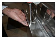
Once all four screws have been tightened, return the server to the upright position, and replace the food pan. Slide the cover back into place, pulling toward you, until the cover is fully returned to place.
