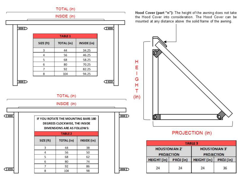
PLEASE NOTE: For Houstonian widths 5' through 8' ONLY (does not apply to widths 3' or 4'), an additional middle support is included in the kit. This middle support is meant to run perpendicular from the wall and can therefore make it difficult or impossible to install around a window/door. Please refer to page 17 in the 5' through 8' width Houstonian owner's manual for more information.
