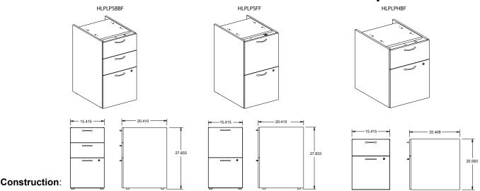
Chassis: 5/8" thick particleboard with double sided melamine surfaces, 0.6mm edgebanding
