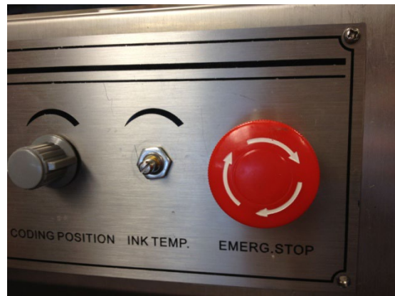
Figure 25. Remove Washer Holding Ink Temperature Potentiometer
