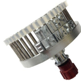
Figure 14. Place silicone pin to lock characters in place.
