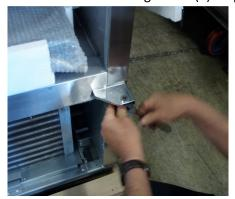
8) You will need to set the new bottom hinge (part# 178HINGCFDBL) to full open, it must spring closed clockwise for door to close properly. Once the hinge is set, install the new bottom hinge.
