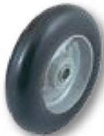
WH 56 8" X 2 1/4" Balloon Cushion 3/4" B.B. 2" Hub Width 450 lbs. Cap. Wt. 4 lbs.
