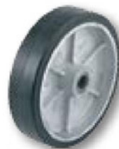
WH 73 8" X 2" M.O.R. 3/4" Roller Bearing 2 1/4" Hub Width 450 lbs. Cap. Wt. 3 1/2 lbs.
