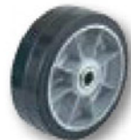
WH 67 6" X 2" M.O.R. 3/4" B.B. 2 1/4" Hub Width 460 lbs. Cap. Wt. 2 1/4 lbs.
