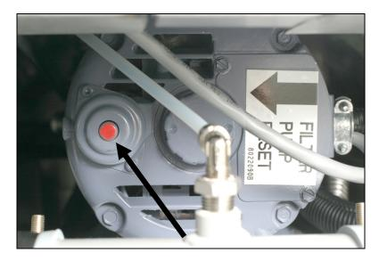
Filter Pump Reset Switch
