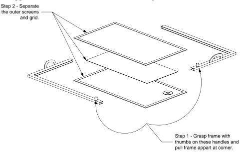
2. Separate the outer screens and grid.
