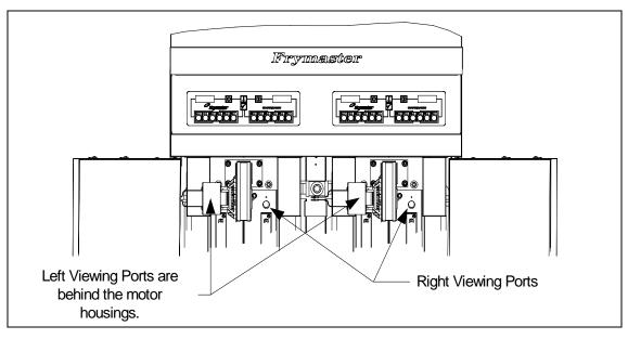
The optimum burn is a bright orange-red glow. If a blue flame is observed, or if there are dark spots on a burner face, adjust the air gas mixture as follows: On the side of the blower housing opposite
