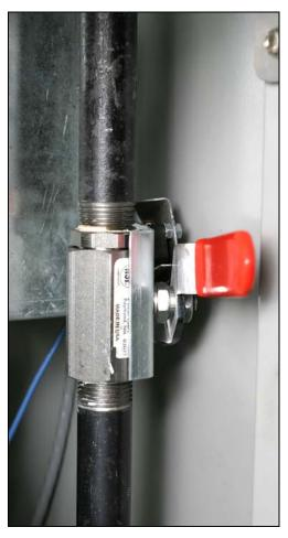
The oil discharge valve handle is shown in the OFF position. Push it down to discharge oil from the filter pan.
