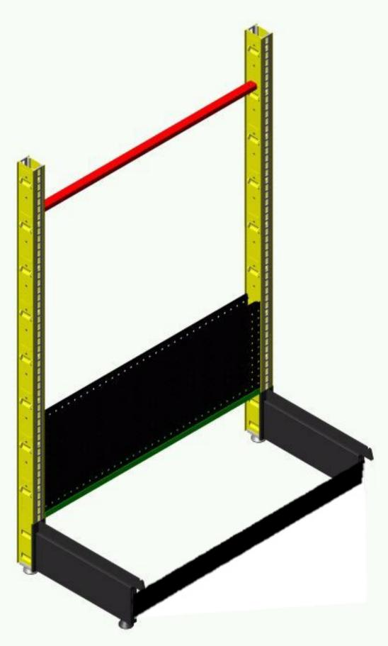
Attach kick pate to the base feet, then install the back panels into uprights.
