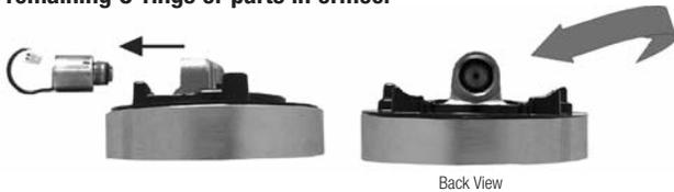
4. Remove black plastic Housing from the threaded end of new Isolated Operator by unscrewing (counterclockwise). It is normal to find fluid inside this housing.
