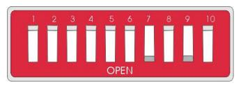
Switch #6 = 5 seconds #7 = 10 seconds #8 = 20 seconds #9 = 40 seconds
