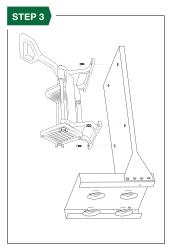
Mount your fry cutter to the countertopmount by screwing it into the back plate.
