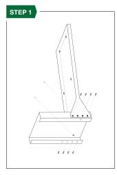
Secure the back plate to the base using the included bolts.
