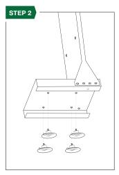
Screw the four suction cup feet into the bottom of the base.
