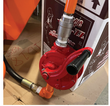
C - With suction tube still inverted, crank oil handle 3–4 revolutions in the direction indicated by the arrow on the pump.
