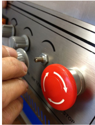
Figure 31. Remove Ink Temperature Knob
