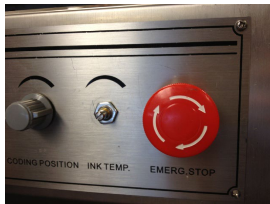
Figure 32. Remove Washer Holding Ink Temperature Potentiometer
