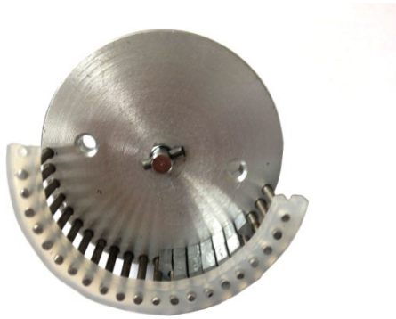
Figure 16. Ensure two holes and pins line up with the base
