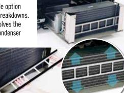
The Clean Sweep<sup>®</sup> Automatic Condenser Coil Cleaner is an electronically controlled brush mechanism that automatically cleans dust and debris from the condenser coil daily, thus maximizing airflow and reducing operating and service costs.
