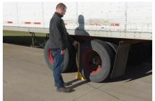
2. Remove the handle from the bumper box. Insert it into the socket on the left side of the leveler plate.
