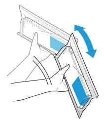
Push all the ink cartridges of the four colors gently into the product until they click in place. Check the color of the ink cartridge label and of the ink cartridge holder label, and set the cartridges to each matching color.
