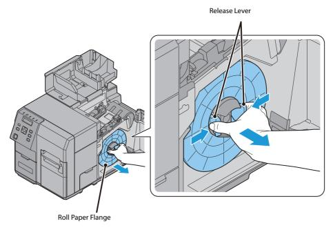
Attach the roll paper to the spindle, and push the core of the roll paper as far as possible so that it is securely fit it into place.
