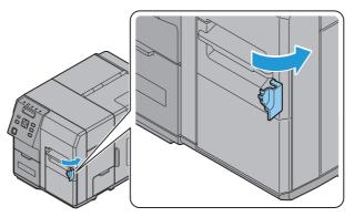
Insert the rewinder's power transmission gear into the cover opening.
