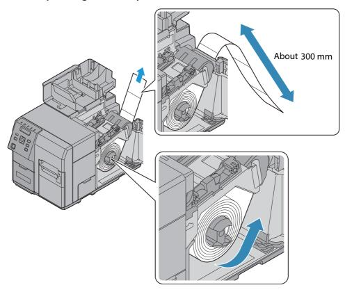
Attach the roll paper flange to the spindle while holding the release lever of the roll paper flange between your fingers. Push the flange to the bottom to align it with the roll paper width.
