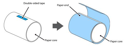
Decide the application position and length of the double-side tape to meet the following conditions. (Recommended tape: Double-sided tape used for starting of winding paper)
