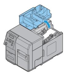
Pull the front cover open lever at the paper feed slot.
