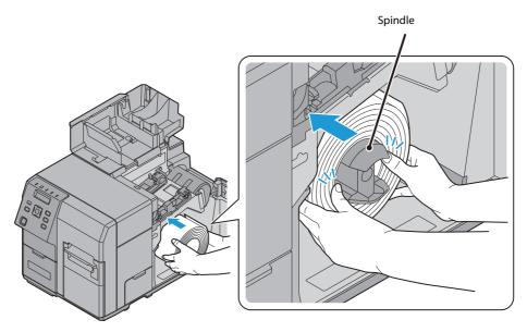
Pull out the end of roll paper about 300 mm {11.8"} in order for the paper auto feeding in the step 12 to go smoothly.
