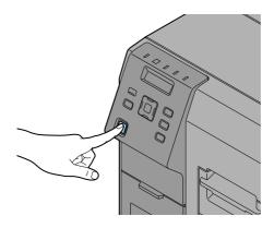
(Power) LED lights up and the power turns on.
