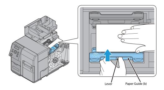
1 Adjust the guide panel of the paper guide (b) so that it aligns perfectly with the edge of the paper.
