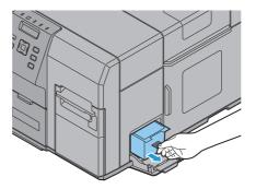
Put the maintenance box into the plastic bag for disposal of used maintenance box.
