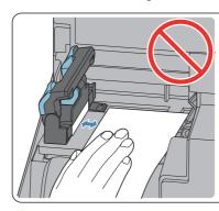
• Do not allow a gap to occur between the guide panel and the edge of the paper.
