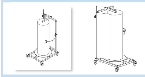
*Note:* Cutter blade cuts paper by sliding down attached cutter rail on the side of the back frame. Corrugated roll can be fed through the gap between the back frame and around the cutter rail.
