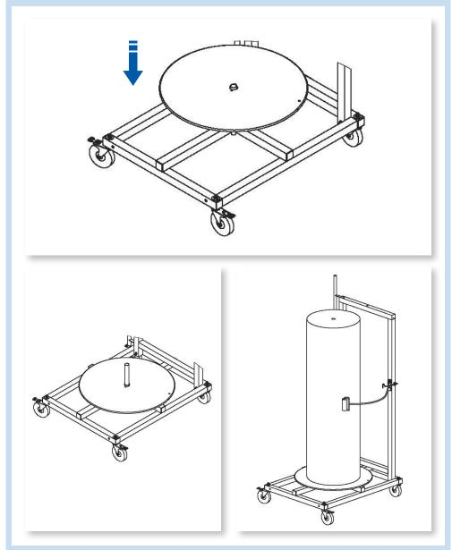
3) Next, slide the dispensing disk over the central cylinder in the middle of the base frame. At this point, the brake arm can be adjusted to size and a corrugated roll can be placed on top of the dispensing disk.
