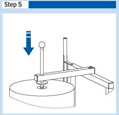
5) Once the top arm is firmly connected, hold bottom core (top) and "o" ring (bottom) in between the corrugated roll and against top arm. Slide adjuster through the designated hole in the top arm and through the core, "o" ring, and corrugated roll.
