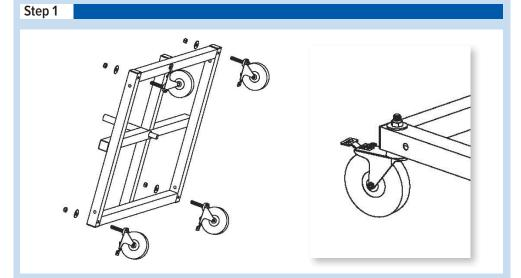
1) Flip the base frame onto its side and slide 5" casters (four) into their designated holes. Using a 3/4" wrench, screw on nylock hex nuts (four) and flat washers into the base frame (four).
