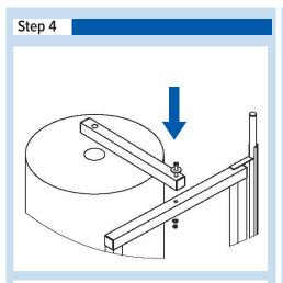
4) To attach the top arm, place on top of back frame and screw in a hex head bolt with flat washer on top and a washer with a nylock hex nut underneath, using a 9/16" wrench.
