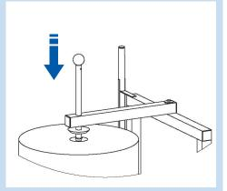
5) Once the top arm is firmly connected, hold bottom core (top) and "o" ring (bottom) in between the corrugated roll and against top arm. Slide adjuster through the designated hole in the top arm and through the core, "o" ring, and corrugated roll.
