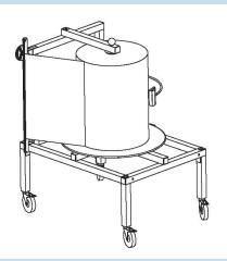
**Note:** Cutter blade cuts paper by sliding down attached cutter rail on the side of the back frame. Corrugated roll can be fed through the gap between the back frame and around the cutter rail.
