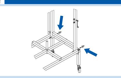
2) Once the base frame is standing, lock the 5" casters in place. Wiggle the back frame into the base frame and attach using 9/16" wrench (two), hex head bolts (two), flat washers (two outside back frame), and washers (two inside back frame). Use synchronized twists on both sides in opposite directions.
