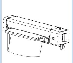
4. Once it is over the outside roller, pull and insert the material into the cutter.
