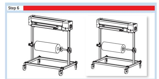
6. Insert one side of the roll onto the core of the Loading Side Brake (#5) and turn the wheel clockwise to extend the arm of the brake to insert into the other the core of the Tension Side Brake (#2).
