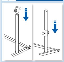
3. Slide one load support (#12) on each vertical side. Lock them in by screwing the knob in, when positioned at half the length of the tube. When assembled, the load supports can be adjusted to accommodate the roll.
