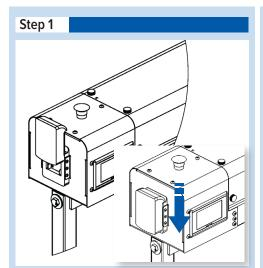
1. Turn on by inserting a fully charged 18-volt battery, and twisting the emergency stop button.
