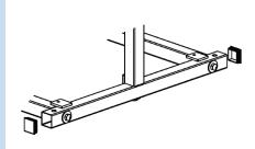
5. Cover the open ends of the bottom side tubes with the provided square tube plugs (#7).
