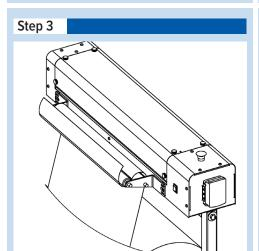
3. Pull the material directly up behind the back roller. Proceed to pull it towards you as you guide it underneath and around the outside roller.
