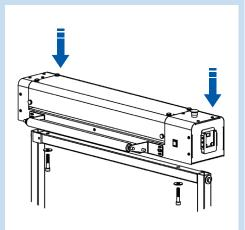
7. With caution, position the automatic sheet cutter (#14) on the top support of the base. Attach the automatic sheet cutter by screwing in the two bolts (#8) and flat washers from the bottom of the top tube to the sheet cutter.
