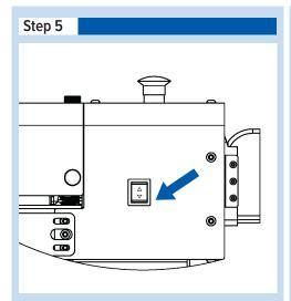
5. When the material is in place, flip the switch back to lower the inside rollers. Let go of the material once the rollers are in place.
