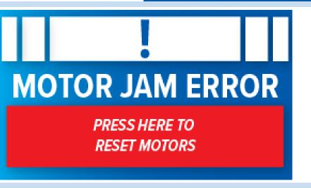
The motor jam error occurs when the material gets caught in the feed rollers or in the cutting mechanism. When this happens, you will get the screen shown above.
