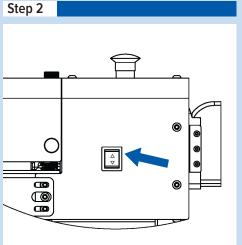
2. Flip the back switch, which raises the inner rollers and is located to the right of the outside rollers.
