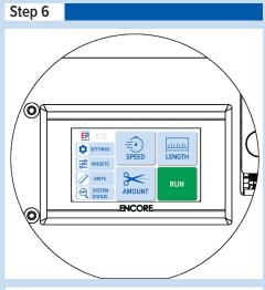
6. Proceed to utilizing the touchscreen to designate the desired unit, speed, length, and number of cuts. Once that information has be set, press Run. Material will now be pulled and cut to the designated settings.
