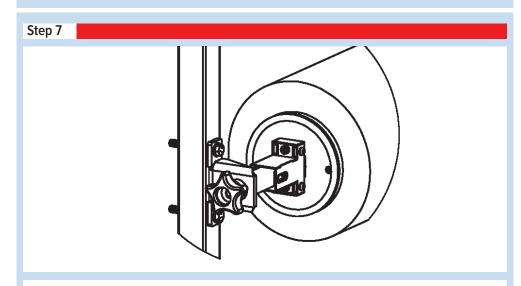
7. Adjust the tension on the roll using the knob on the Tension Side Brake (#2) as needed, turning right to increase tension and left to decrease.
