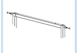
4. Attach the top support weldment (#3), with the flat washers and screws that are included. The plates should be parallel to the side of the vertical tubes when attached.
