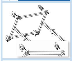
6. Carefully put the stand on its side so that the top support is touching the ground. Proceed to screw in the 5" casters (#9) to the bottom of the side frames by using the flat washers, and nylon nuts (#10). When attached, carefully, turn the stand back to its proper stance with the casters on the ground.
