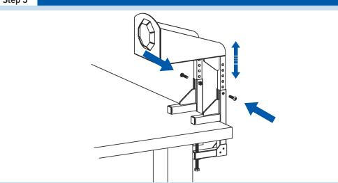
3. The height of the dispenser can be adjusted by removing the two screws (#7) and sliding the chute up to the desired length. When chosen, secure in place by screwing in the two screws (#7) that were removed.
