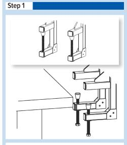
1. Loosen the two bolts (#3) to thickness of the work bench being used. Push onto the work bench once bolts are loose.
