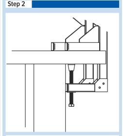
2. Tighten the bolt to secure dispenser onto the work bench.
