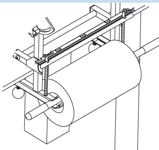
5. Attach the support tube with the kraft paper roll on to the EP-5955.
