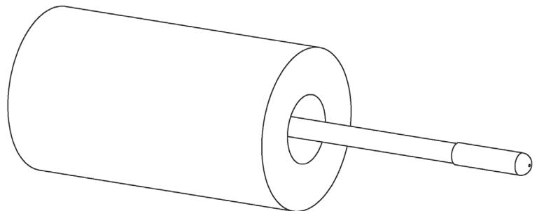
2. Insert the support tube into the kraft paper roll.
