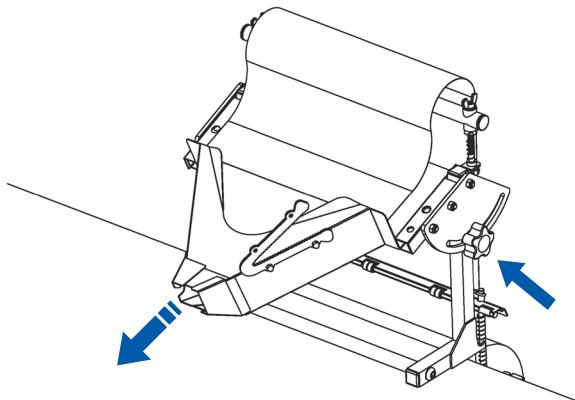
8. Feed the paper through the chute and use the cutter to cut paper to desired length. Adjust the positioning of the dispenser as needed by unscrewing the pivot plate knob enough to swing the chute into the position needed then secure in place by screwing in the knob.
