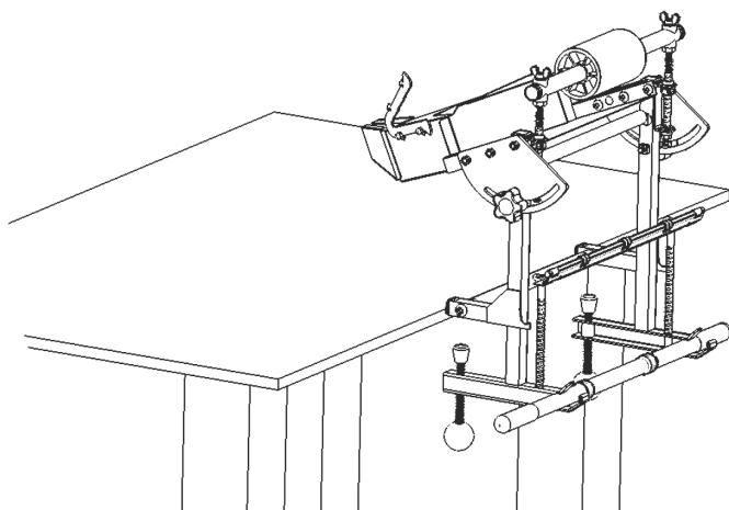
3. Slide the dispenser onto the table, up to the upright tube of the side support weldments so it is fully against the table.
