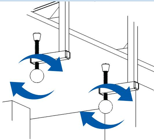
4. Tightly screw the ball knob handles up against the bottom of the table to securely mount the dispenser.
