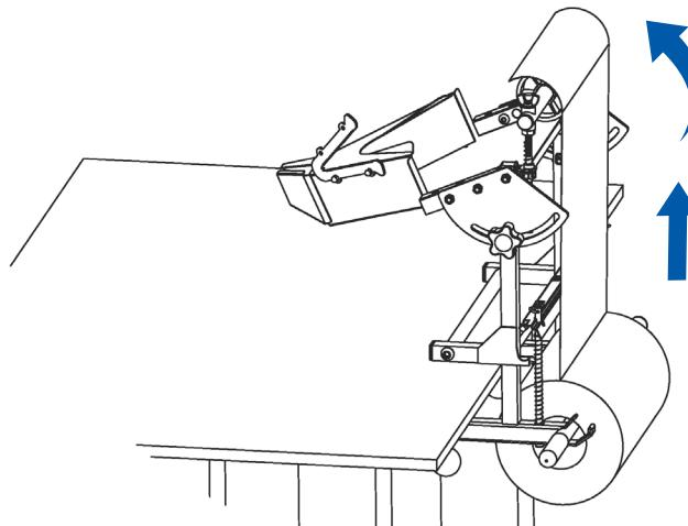
6. Pull kraft paper under the brake strip and over the PVC roller.
