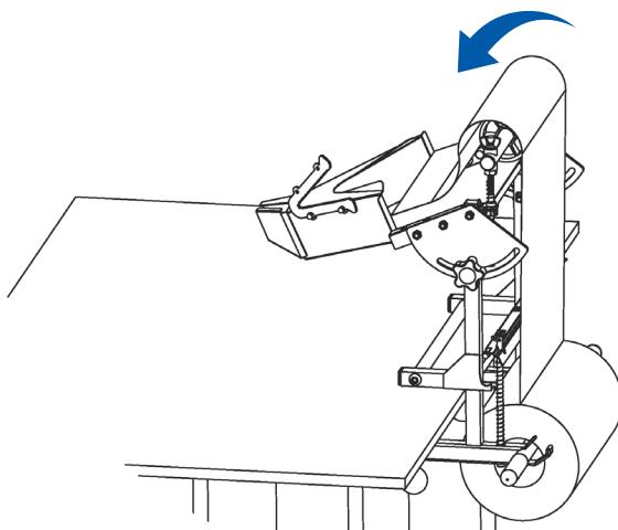
7. Wrap kraft paper under the PVC roller and feed the paper towards the chute.
