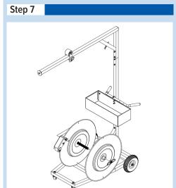
7. Unscrew the Wing Nut and remove the Front Disk Assembly.
