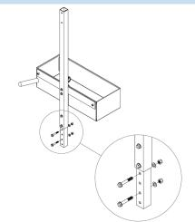
1. At the bottom of the Mast Assembly remove the two Hex Head Bolts, along with the Washers, and Nylock Hex Nuts.
