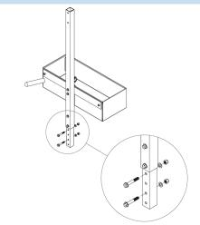
1. At the bottom of the Mast Assembly remove the two Hex Head Bolts, along with the Washers, and Nylock Hex Nuts.
