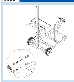
2. Slide the Mast Assembly into the square beam on the Base Weldment and replace the two Hex Head Bolts, Washers, and Nylock Hex Nuts.
