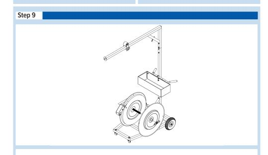
$9. \, \mbox{Slide}$  on the Front Disk Assembly and replace the Wing Nut to secure the coil.
