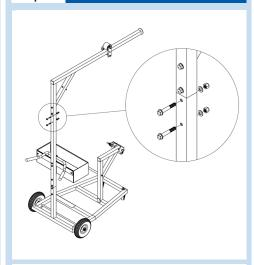
4. Slide the Suspension Beam into the top of the on the Mase Assembly and replace the two Hex Head Bolts, Washers, and Nylock Hex Nuts.
