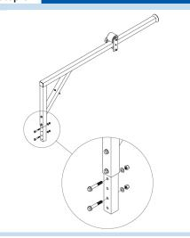
3. At the bottom of the Suspension Beam remove the two Hex Head Bolts, along with the Washers, and Nylock Hex Nuts.
