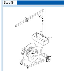
8. Load a Poly or Steel strap coil – make sure the orientation allows for counterclockwise dispensing through the Brake Assembly.
