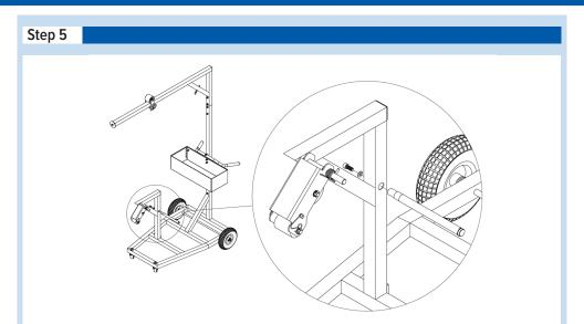
5. On the left side of the Disk Stand, unscrew the Socket Head Screw and remove the 3/8" Split Lock Washer. This will release the Retaining Ring on the other side.
