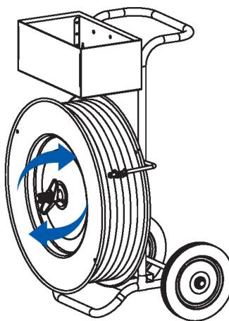
3) Release brake arm and reload the front disk. Twist the wing nut back onto the spindle. Make sure the strap is secured between the two disks.
