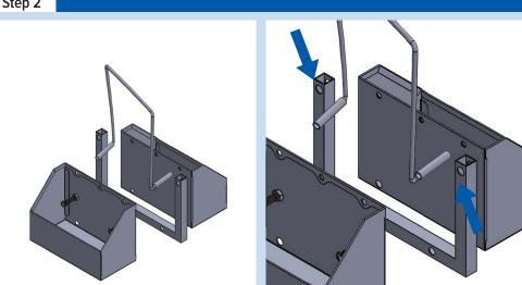
2. Then, slide tubes on the handles and finally slide the handle through the middle support holes.
