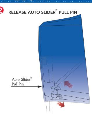
With one hand, slighty push up on the truss near the **Auto Slider® Pull Pin** to relieve pressure.
