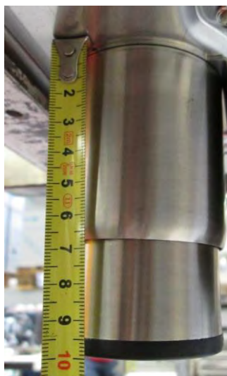
Fig. 55: Making sure that the feet are at the same height
