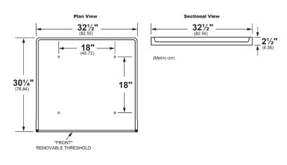
General: Furnish and install as shown on plans DURAPAN™ Wash Machine and Water Heater Pan, Model 98, as manufactured by E.L. Mustee & Sons, Inc. One-piece compression molded fiberglass using matched metal molds under extreme heat and pressure. Shoulder will be no less than 2 1/2" high. Removable threshold with water tight seal secured by stainless steel screws. May be secured to sub-floor; mounting hardware provided. Shall include (1) 1" NPSM-90° elbow fitting. Color: White.
