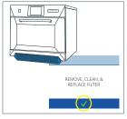
Remove the air filter and wipe it clean or wash in soapy water. Dry and replace and then press the green tick to continue.
