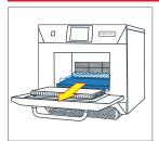
1. Remove the oven rack and base plate.
