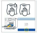
Remove the Merrychef cleaner with a clean wet cloth. The door seal can also be gently wiped if necessary to remove food debris.
