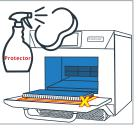
Apply oven protector (optional). Spray Merrychef Protector onto a sponge and spread lightly onto the sides of the inside of the oven, the back, the base, the roof and the oven door and heat oven afterwards.
