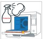
7. Apply oven protector (optional). Spray Merrychef Protector onto a sponge and spread lightly onto the sides of the inside of the oven, the back, the base, the roof and the oven door and heat oven afterwards.
