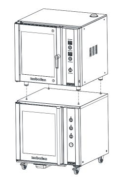
Lower E35 Oven onto P85 Proofer, aligning Oven Stacking Pins with oven legs.
