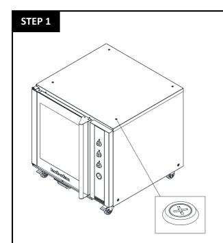
Remove 4 blanking screws and cup washers from P85 Proofer top cover panel.
