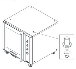
Fit 4 Oven Stacking Pins supplied as shown.
