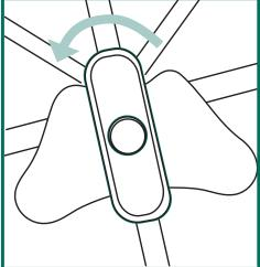
Adjustment: Turn the top knob counterclockwise to adjust the dish dolly arm location.
