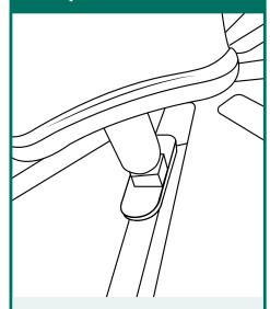
Insert the dish dolly arm into its desired slot.
