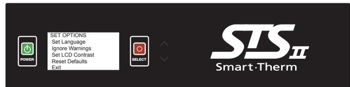
3. Use the **UP/DOWN** arrow keys to move the caret symbol (>) to the desired option, and press **SELECT**.
