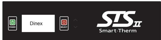
1. The unit must be powered down with Dinex in the display. Press and hold the **SELECT** key for 7 seconds.
