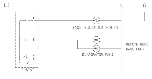
NOTE: Provided with 6.00" (15cm) leads from junction box for field connection.
