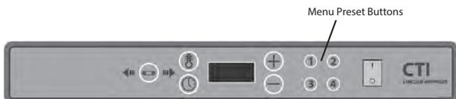
2. Press and release the menu button again to reach the time/belt speed setpoint. The display will flash the time/belt speed setpoint. Press the (+) or (-) button to reach the desired time/belt speed.
