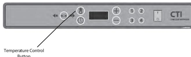
4. Press and release the temperature button again to leave manual mode and activate the manual settings.
