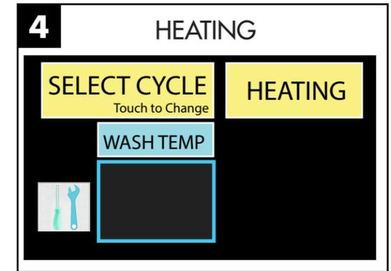
'HEATING' appears after the fill. Machine preheats for 15-20 minutes.
