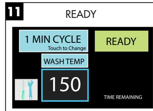
'READY' appears at the end of the cycle. Open the door and remove the clean wares.
