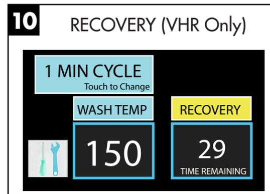
'RECOVERY' appears as heat and steam are removed from the wash chamber.
