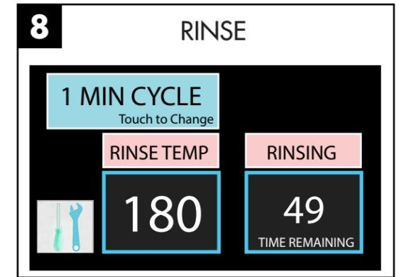
Monitor the final 'RINSE TEMP' to ensure it maintains a minimum of 180°F during the final rinse.
