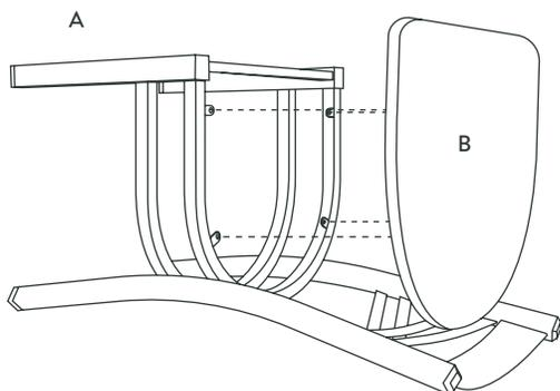
**Option 2:** Place seat (B) upside down on a flat surface, preferably a table. Align chair frame (A) on top of seat (B). Center seat with four screw holes on frame, push seat against the back of the frame and ensure front of seat is parallel to the front of the frame.
