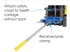
**Step 4**: Raise the forks only as high as necessary to lift the roll of carpet off of the ground and to avoid contact with objects during transport. DO NOT leave a raised roll unattended. Always unload the carpet pole before leaving the forklift.
