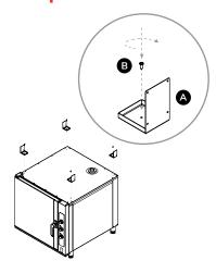
Attach the 4 L-brackets (A) to the top of the bottom oven with 1 screw (B) each. Ensure the vertical side of each L-bracket is facing out as shown.
