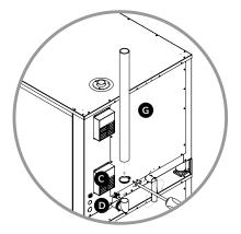
Connect the long exhaust pipe (G) to the 90-degree pipe fitting (D) installed in Step 4. Use 1 screw clamp (C) to secure.
