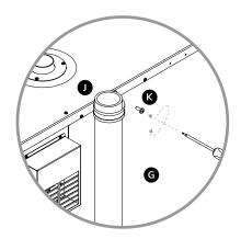
Feed the long exhaust pipe (G) through the exhaust pipe holding bracket (J). Use the holding bracket set screw (K) to secure it to the back of the top oven as shown.
