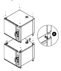
Ensure the legs are installed on the combi oven unit being stacked on top. With the help of another person, lift the top combi oven onto the bottom combi oven. Place the legs onto the L-brackets (A) as shown. The feet should fit inside the L-brackets.
