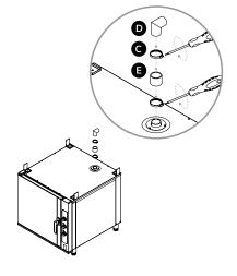
Place the short exhaust pipe (E) and a  $90^{\circ}$  pipe fitting (D) over the steam exhaust vent, ensuring the  $90^{\circ}$  pipe fitting (D) is facing the back of the combi oven as shown. Use 2 screw clamps (C) to secure.
