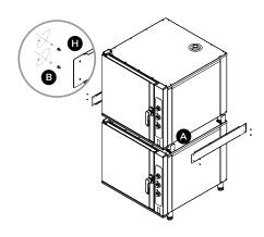
Attach the 2 side brackets (H) to the sides of the combi ovens where they meet. Use 4 screws (B) on each side to secure the side brackets (H) to the L-brackets (A) as shown.
