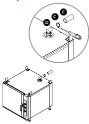
Connect the medium exhaust pipe (F) to the 90-degree pipe fitting (D) installed in Step 2. Use 1 screw clamp (C) to secure.
