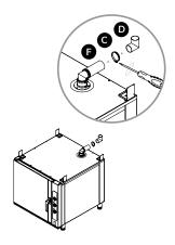
Connect the remaining  $90^{\circ}$  pipe fitting (D) to the medium exhaust pipe (F), ensuring it is facing directly up as shown. Use 1 screw clamp (C) to secure.
