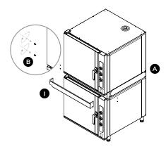
Attach the front bracket (I) to the front of the stacked combi ovens and use 4 screws (B) to secure to the L-brackets (A) as shown.
