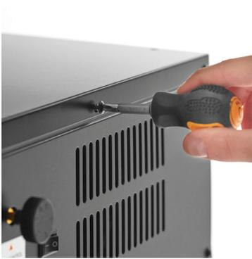
2. Unscrew the (3) screws on the back of the unit connected to the top panel.
