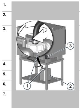
Remove the screw closure (1) with the connected tube from the grease collection canister (2).
