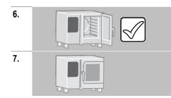
Check to make sure that the suction panel is installed properly:The suction panel is in place and locked into place at the top and bottom.
