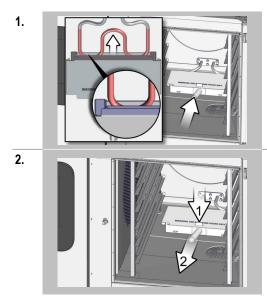
Grab the smoker box containing the bisquettes from the handle and slide it all the way onto the smoker heater inside the oven cavity. Make sure that the heating element goes into the smoker box opening meant for the smoker heater.
