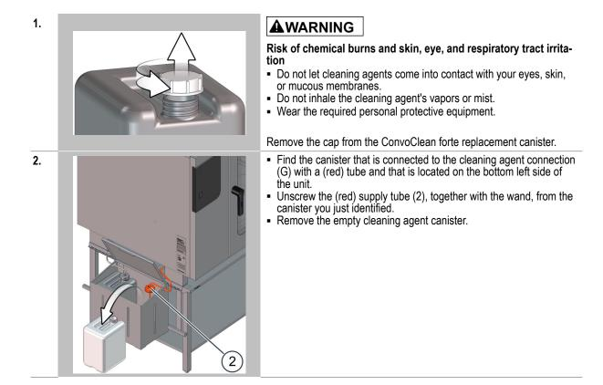
Put the new, full canister (1) containing cleaning agent in place.
