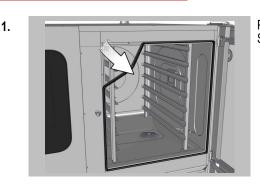
Pull out the hygienic plug-in gasket around the unit door opening. Start from the corners.
