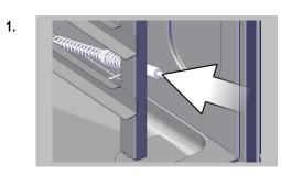
Slide the core temperature probe into the spiral holder on the righthand side rack.
