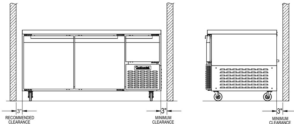
and strong enough to support the total combined weights of your new model plus the maximum product load which might be placed into it. Keep in mind that all the weight is concentrated at the caster or leg locations. To estimate the possible product weight, assume that each cubic foot of storage space weighs approximately 35 pounds. Multiply 35 pounds by the amount of cubic feet in the cabinet to obtain the product load weight.
