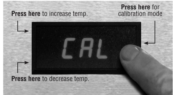
For example, if the sensing device in the cabinet reads 38° and the thermometer display reads 40°, press on the lower left corner twice so that “-2” appears on the display. After adjusting the offset, press on the right center of the display again to exit calibration mode. Wait 10 to 15 seconds for the cabinet temperature to be displayed and recheck the calibration.
