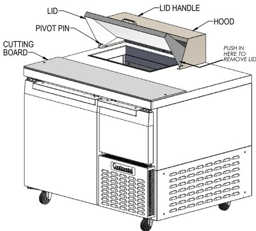
**IMPORTANT NOTE:** The top opening on your sandwich top must be completely filled with pans at all times, even if some pans are empty, to maintain air flow for proper cabinet and pan temperature.
