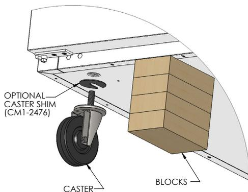
**Do not attempt to level casters by unscrewing them from the cabinet and leaving them loose, as this will cause damage to the cabinet and leg hole threads, voiding all warranties.**
