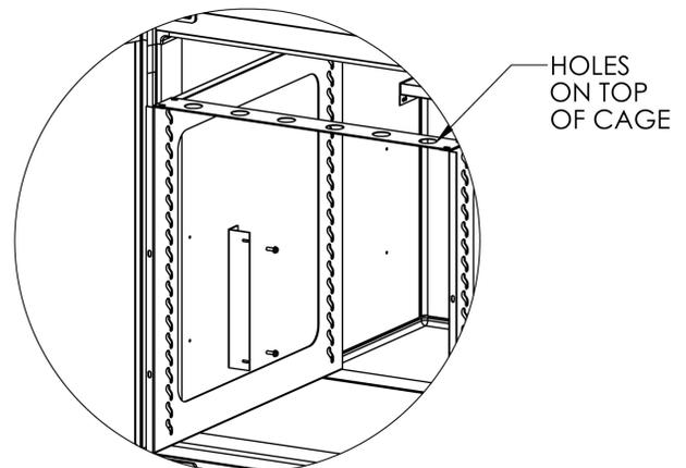
FIGURE 18A: Pan Slide Cage - Center Bracket
