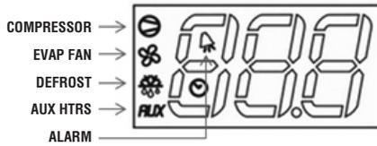
The control icons shown above will be illuminated when the associated function is active. If an icon is flashing, it means the function will be activated after the controller delays are finished.
