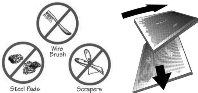
**DO NOT USE:** abrasive cleaners, steel pads, wire brushes, scrapers or knives to clean your equipment.
