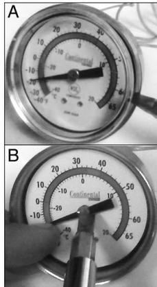
Use a small straight-blade screwdriver and place on center slotted hub of thermometer. Carefully hold the needle and turn the center screw clockwise to lower and counterclockwise to increase the desired temperature, as shown (see **Photo B**). Replace the lens cover and recheck the calibration.
