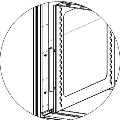
FIGURE 18C: Pan Slide Cage - Install Angle Slides
