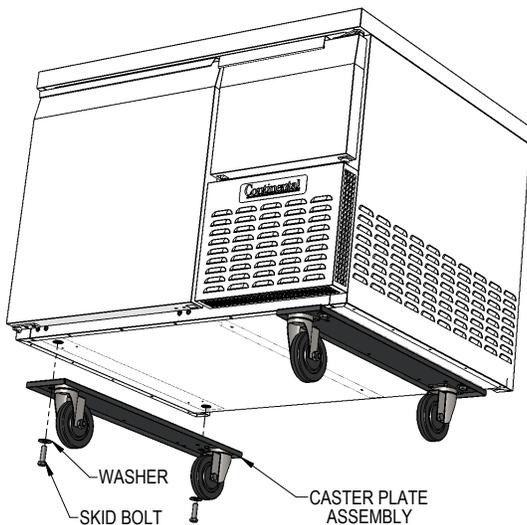
Using the small holes in the plate as a template, drill 1/8" pilot holes in the bottom of the cabinet. (**Note: drill only until you penetrate the metal bottom of the cabinet. Do not continue to drill into the insulation, or you may damage the cabinet.**) Secure the caster support plate assembly to the cabinet with a sheet metal screw in each of the drilled holes. Tighten the 1/2" bolts. Repeat these steps to attach the other plate assembly to the opposite end of the cabinet.
