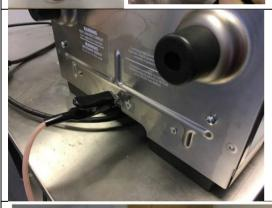
Wait 5 Minutes to allow the capacitor tonaturally discharge its energy.
