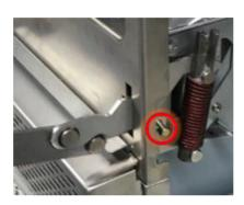
**5.** Open the door and fit the locking pins in place to prevent the hinges snapping back.
