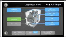
3. Remove the air filter at the front of the oven. The colour of the air filter symbol on the display should change from grey to green indicating that the microswitch circuit for theair filter is operating correctly. Replace the air filter and the colour should change back to grey.
