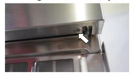
**1.** Remove the two M4 x10 hex Head Flange Bolts on the bottom of the door.
