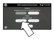
Menus can also be downloaded onto the oven through settings / updates, without the need to turn off the oven first.
