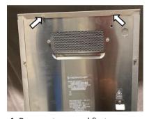
**1.** Remove top panel first. Unfasten the M5.5 hex head flange bolts at the back panel of the appliance attaching the top panel to the back panel.
