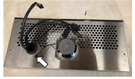
4. Unfasten the three Posidrive screws at the bottom of the removed front panel and un-slot from the top of the panel to separate from the metalwork.
