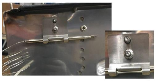
The cavity overheat thermostat switch is located at the rear of the oven, mounted on the left-hand side of the magnetron air flow ductwork, fitted by two M3 x 4 CSK Philips SS Screws and flat washers torqued to 1Nm.
