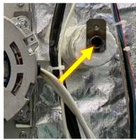
The straight steam vent runs from the rear of the cavity directly out of the rear of the oven, secured by a single M4 flange nut and gasket torqued to 2.1Nm. The steam vent is further supported by connection to the rear panel.
