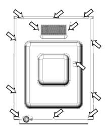
Overview of all M5.5 hex head flange bolts securing the panels of the casing.
