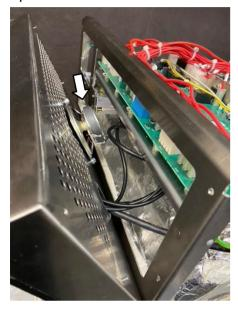
The speaker is located on the rear of the front panel, behind the UI, by two M7 hex nuts and connected directly to the UI loom.
