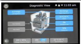
2. Select a component symbol to switch on (red). Select again to increase the level (remains red) or turn off (blue). Exceptfor the magnetron(s), all the component tests will work with the door open or closed.
