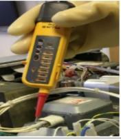
Re-test your proprietary voltage tester is working correctly and test to ensure the capacitor is discharged(dead) at the magnetron(s) and the HV transformer(s).
