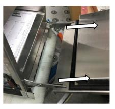
**6.** Slide door off the hinges to remove.
