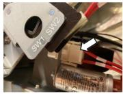
**1.** Unplug the electrical connection of the cooling fan on the right-hand side of the appliance.
