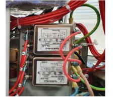
2ph ovens, L1 & N connected to bottom filter, live on the top terminal, neutral on the bottom terminal. L2 connected to the top filter (top terminal) and neutral linked from bottom filter.
