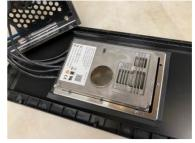
5. Unfasten the eight posidrive screws from the UI clamp to separate the UI from the glass panel.
