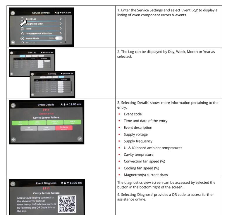
Further details can be read by copying the event log to a USB and opening the files on a computer.
