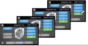
5. Select the cooling fan and check if it is operating correctly.
