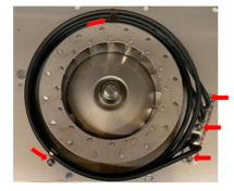
The element is fixed using two M7 hex bolts on the X12 & three on the X16, tightened to 2.1 Nm and supported with a single M5.5 hex flange nut on the X12 & two on the X16, tightened to 1.7 Nm.
