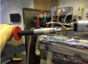
Hold the probe against the HV capacitor terminal for 5 seconds, removing any covers to do so. Repeat on the other set of terminalson the same capacitor. Repeat this process on both HV capacitors for equipment with two magnetrons.
