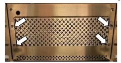
The rear air diffuser plate in the cavity prevents large foodstuff from hitting the rear of the cavity. Loosen the bottom two M7 hex nuts and unfasten the top two M7 hex nuts to remove/refit.
