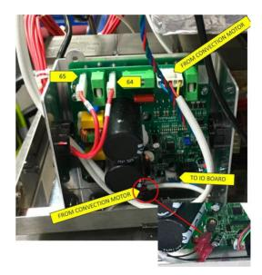
**Note:** Ensure the replacement board has a jumper (link) fitted to the J5 position.
