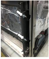
**4.** Unfasten and remove the four M5 flange locking nuts & M5 hex head bolts from the door hinges
