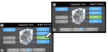
6. Select the convection fan and check if it is operating correctly.
