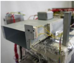
The manual reset button is now directly accessible from the rear of the oven.
