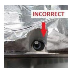
Ensure the flange nuts holding the convection motor in place have been torqued to 2.1Nm and are torqued diagonally and not clockwise.
