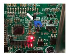
Link positions are factory pre-set based on the model of convection fan used in the conneX ovens. The link positions must not be altered without express instruction from Merrychef.
