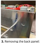
Unfasten the six M5.5 hex head flange bolts attaching the back panel to the cooling duct (two bolts), the exhaust pipe (one bolt) and the base plate (three bolts) of the appliance. Move the back panel up to remove
