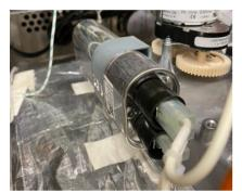
The high voltage capacitor is located on top of the cavity and is fixed by a sheet metal bracket and a pozidriv (PZ2) screw
