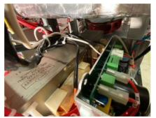
The X12 standard power variants have a single HV transformer at the rear of the oven, under the cavity.
