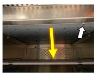
7. Remove & refit upper impinger plate inspecting for cleanliness and signs of damage (if required follow the instructions laid out in the replacement impinger Kit). Visually check the partition plate for signs of discolouration or damage.
