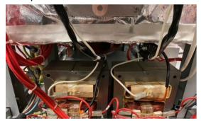
The X16 has two HV transformers, side by side, at the rear of the oven, under the cavity. The right-hand transformer is for the right-hand microwave circuit & components.
