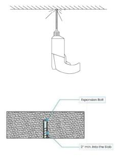
4. Drive the expansion screw, screw in the threaded rod, and then screw in the four Nuts, where nut 3 is next to nut 4. The position of each screw should be at the same height from the ceiling.
